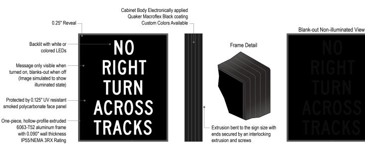
Outdoor/indoor blank-out signs with an aluminum cabinet, backlit white or colored LEDs and contrasting black face The sign message is formed by a black opaque printed face with stenciled areas that illuminate when activated and blank-out when deactivated
