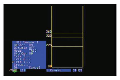
extension to add to each output. This extension is for each trip line, and is equal to the amount of time it takes for a vehicle traveling over the maximum speed noted to get to the next trip line.
