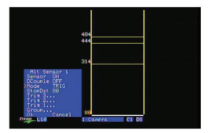
The image to the right from the Vector setup screen shows the 50 mph max speed setting for trip line 1 at 314 feet.
