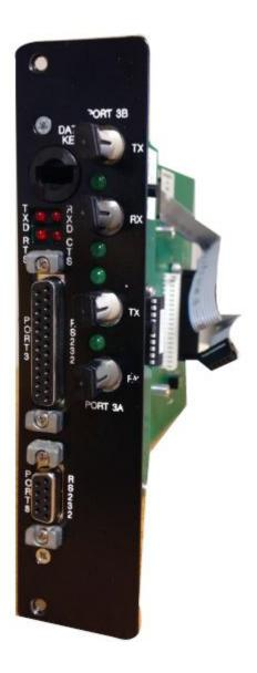
The Fiber Optic port consists of two fiber optic receivers, logically connected to the NEMA Port 3. Data received on either fiber optic receiver is sent to the controller, as well as the other fiber optic transmitter. The Fiber Optic acts as a repeater, receiving controller data, plus boosting and retransmitting the signal to the next controller. If received message is destined for this controller, the controller reply is transmitted simultaneously on both fiber optic transmitters.
