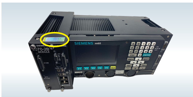
Product Label placement on all controllers containing the ATC Cabinet Compatible Backplane
