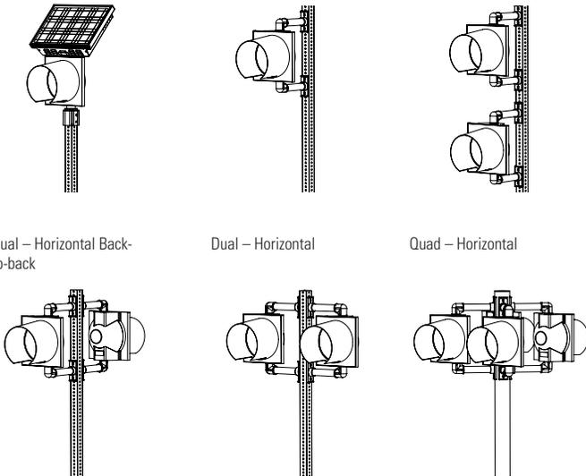
\* Other solar engine and beacon mounting configurations are available.
