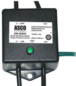
The **ASCO Model 235** surge protector is a compact submersible device that is designed to be installed directly within a light pole to help protect the sensitive lighting ballast and power supply from damaging transients. Model 235 easily fits into the 3 in. x 5 in. hand hole located at base of the light pole and is wired in series with the load.
