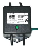
The **ASCO Model 235** surge protector is a compact submersible device that is designed to be installed directly within a light pole to help protect the sensitive lighting ballast and power supply from damaging transients. Model 235 easily fits into the 3 in. x 5 in. hand hole located at base of the light pole and is wired in series with the load.
