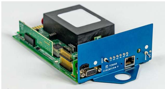
4140 Version 2, four channel, wide panel, optical signal processor with Integrated Confirmation, event logging, and Ethernet port
